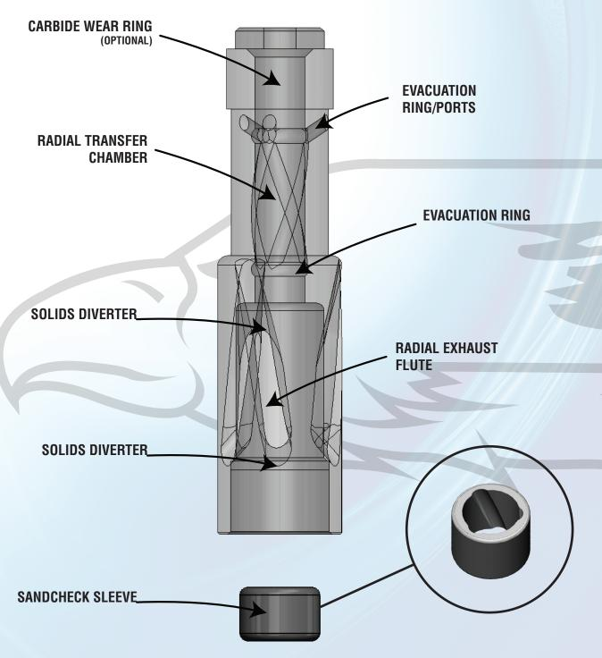
Material Construction: 316 Stainless Steel Nickel Carbide
